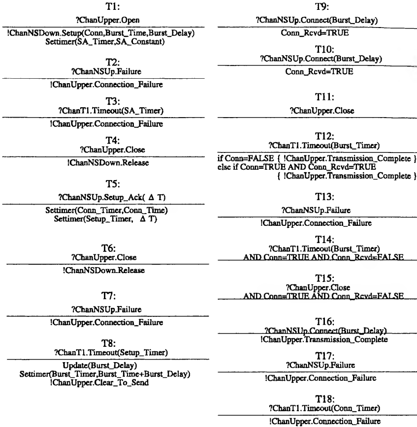
Fig. 4. State transitions for source client.
