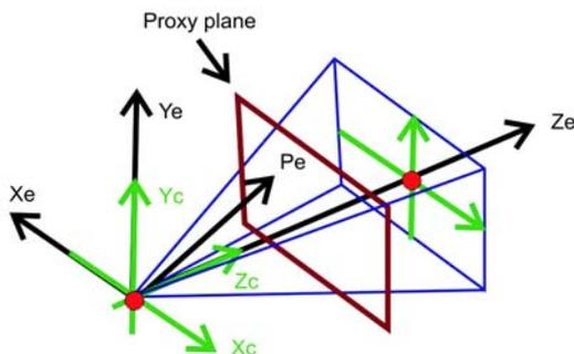
Fig. 6. Camera location in the eye coordinate system.
