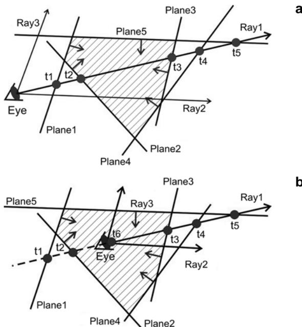
Fig. 7. Determination of start and end points. The viewpoint outside (a) and inside (b) the clipped volume.
