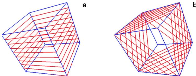
Fig. 1. Axis-aligned (a) and view-aligned resampling slices (b).
