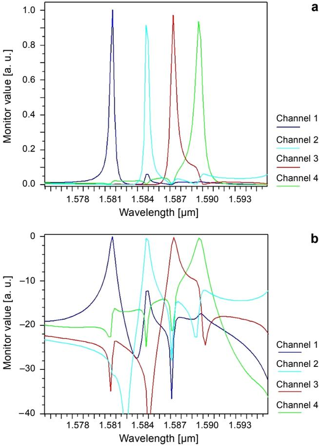
Fig. 7. The output spectra of the proposed demultiplexer. Linear (a) and dB (b) scale.
