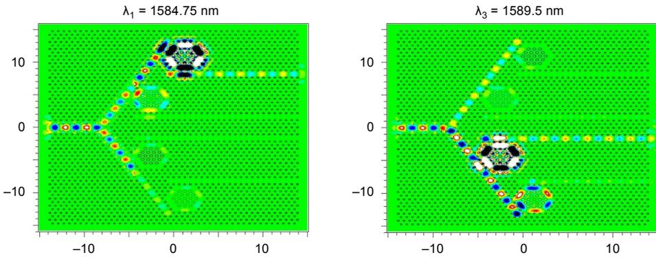
Fig. 8. The electric field distribution of the proposed demultiplexer.
