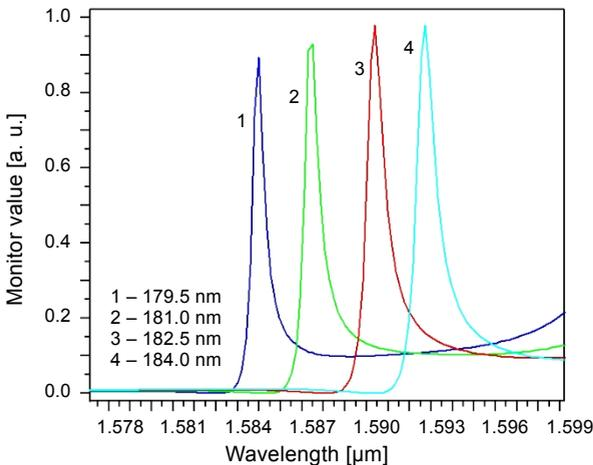
Fig. 5. The output spectra of the proposed filter for different values of  $R_1$ .
