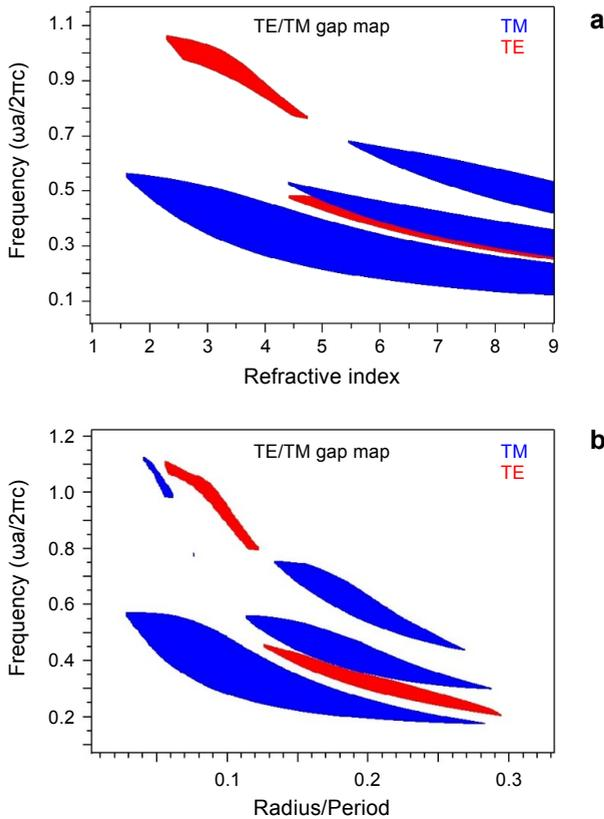
Fig. 1. Gap map diagrams: variation of PBG versus refractive index (a) and  $R/a$  ratio (b).
