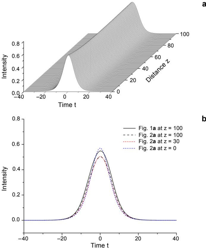
Fig. 2. The evolution plot of the solitary wave with amplitude perturbation (a). The compared plots at different transmission positions (b).
