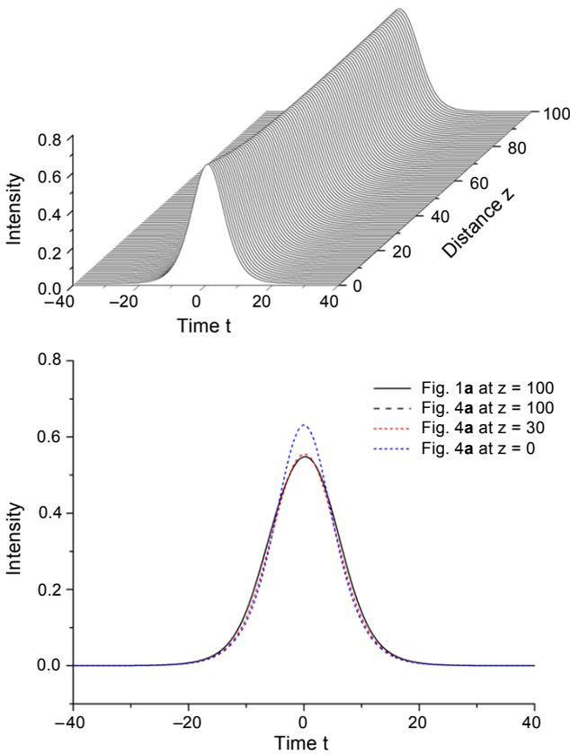
Fig. 4. The evolution plot of the solitary wave with phase perturbation (a). The compared plots at different transmission positions (b).
