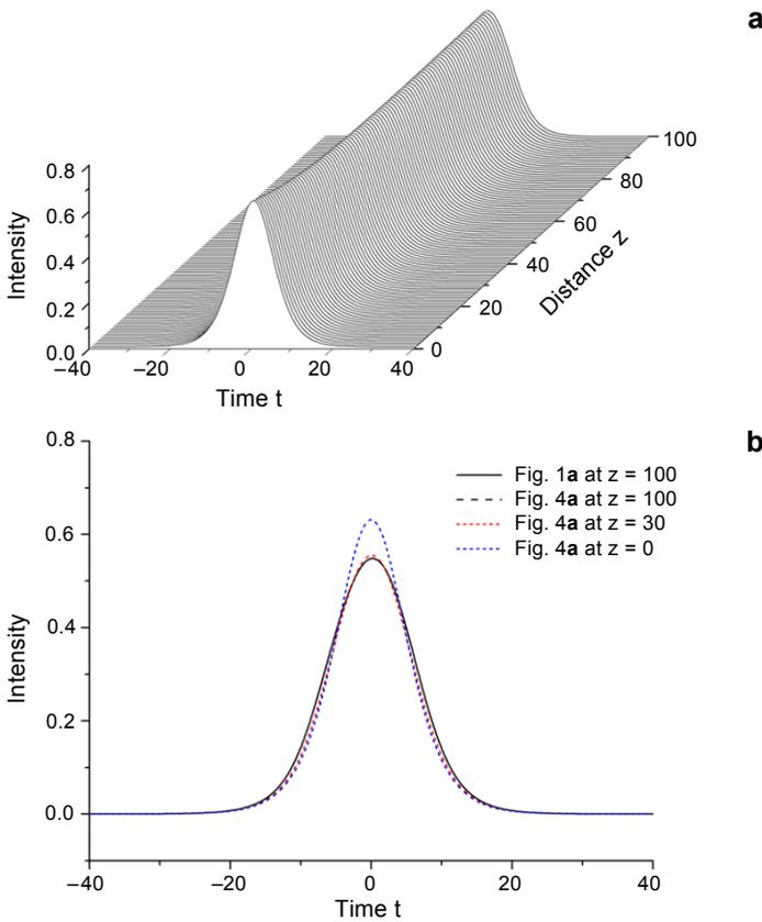
Fig. 4. The evolution plot of the solitary wave with phase perturbation (a). The compared plots at different transmission positions (b).
