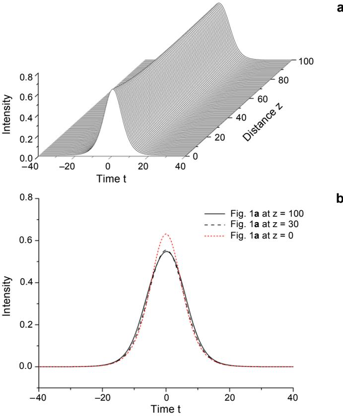
Fig. 1. The evolution plot of the solitary wave (a). The compared plots of the initial pulse at different transmission positions (b).
