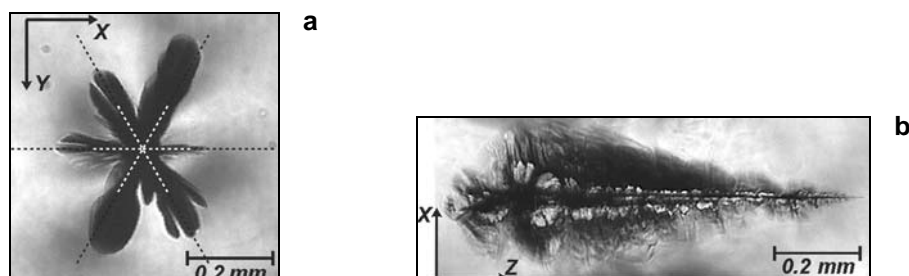
Fig. 1. View of the damage tracks for Z-cut LN crystals (a) and the same damage track observed from Y-plane (b). The light propagates along the Z axis.
