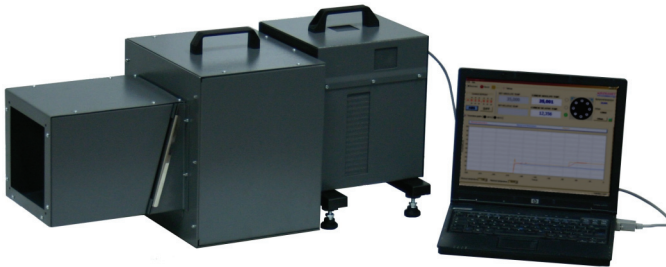
Fig. 7. Photo of the test system for testing passive surveillance THz imagers.
