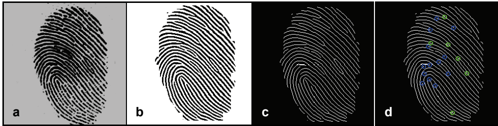
Fig. 10. Results of algorithm based on Hong filtration [12]. Filtered image (a), binarized form (b) and thinned form (c) with marked minutiae inside ROI (d).
