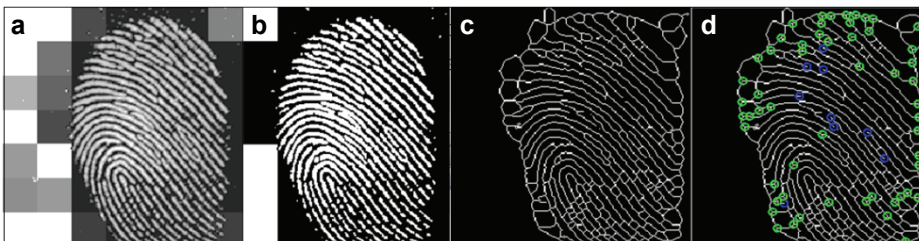
Fig. 8. Results of algorithm based on Fourier filtration [12]. Filtered image (a), binarized form (b) and thinned form (c) with marked minutiae inside ROI (d).
