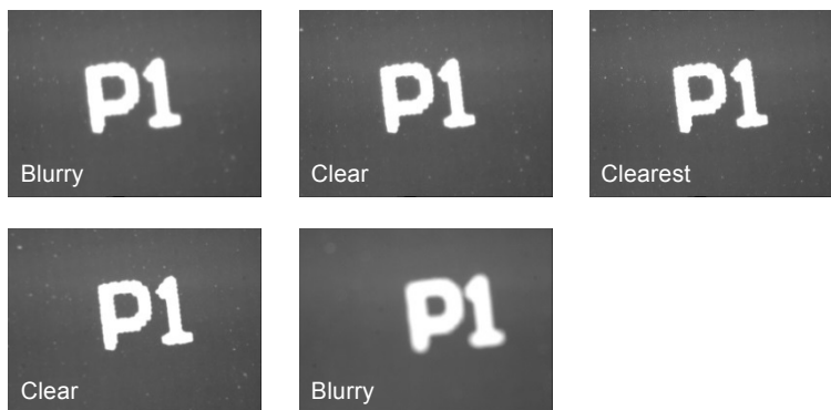
Fig. 2. Partial calibrated left views of stereomicroscopic image sequence.
