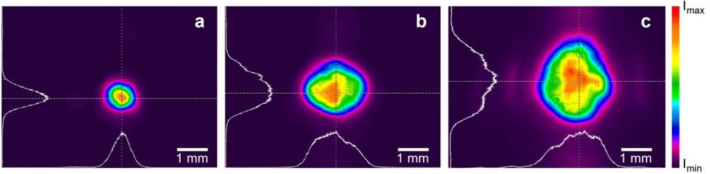
Fig. 2. The output laser beam patterns. Output beam patterns for the diameter of the limiting spatial filter are set to be (a) 1 mm, (b) 2 mm, and (c) 7.5 mm.
