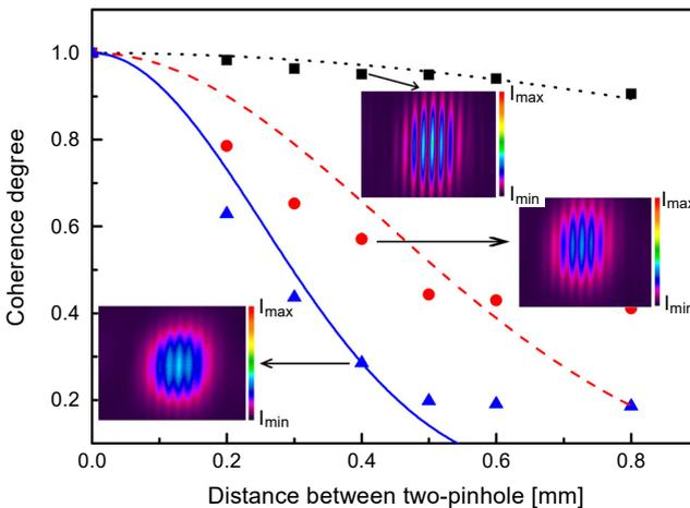
Fig. 7. The degree of coherence as a function of the distance of the two-pinholes for three different diameters of the spatial filter. The black squares with dotted line denote the result for a spatial filter diameter of 1 mm, the red circles with dashed line denote the result for a spatial filter diameter of 2 mm and the blue triangles with solid line denote the result for a spatial filter diameter of 7.5 mm.
