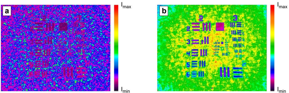
Fig. 5. Experimental demonstration of low-speckle imaging by using laser beams with different coherence. (a) The diameter of the limiting spatial filter is  $d = 1$  mm, and the spatial coherence of the output laser beam is high. (b) The diameter of the limiting spatial filter is  $d = 7.5$  mm, and the spatial coherence of the output laser beam is low. The speckle is largely reduced.
