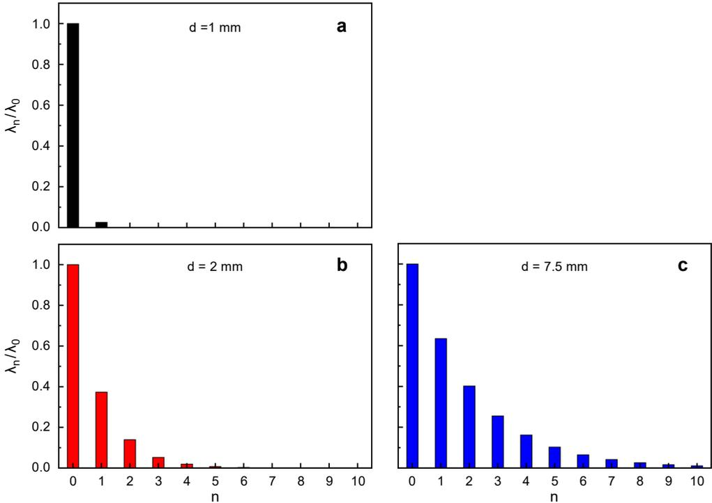
Fig. 8. Distribution of transverse modes. The diameter of spatial filter is set to: (a)  $d = 1$  mm, (b)  $d = 2$  mm, and (c)  $d = 7.5$  mm.
