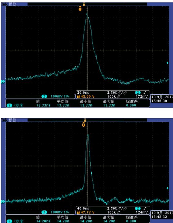
Fig. 3. The pulse shapes of the *Q*-switched laser. (a) The diameter of the limiting spatial filter  $d = 1$  mm, the pulse width is 13.3 ns, (b)  $d = 2$  mm, and the pulse width is 14.2 ns, (c)  $d = 7.5$  mm, and the pulse width is 16.4 ns.
