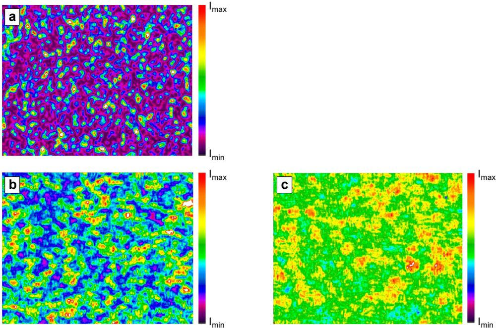
Fig. 4. The speckle patterns of the output laser light are detected by a CCD camera. (a)  $d = 1$  mm,  $C = 0.929$ , (b)  $d = 2$  mm,  $C = 0.574$ , and (c)  $d = 7.5$  mm,  $C = 0.184$ .
