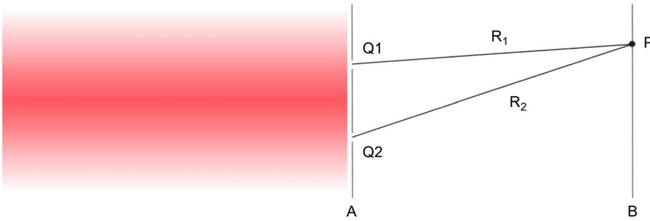
Fig. 6. Notation relating to Young’s two-pinhole interference experiment for measuring the degree of coherence of the output laser beam.
