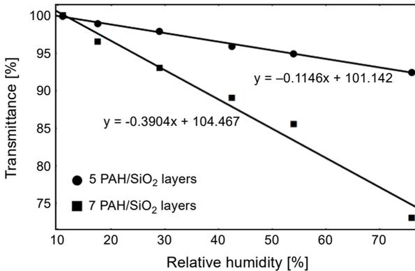
Fig. 4. Transmittance vs. relative humidity. The curves of a POFHS coated with five and seven PAH/SiO<sub>2</sub> layers. Calculations were for the wavelength of 611 nm, for the core diameter of 190 μm and for 30 mm long sensitive region.
