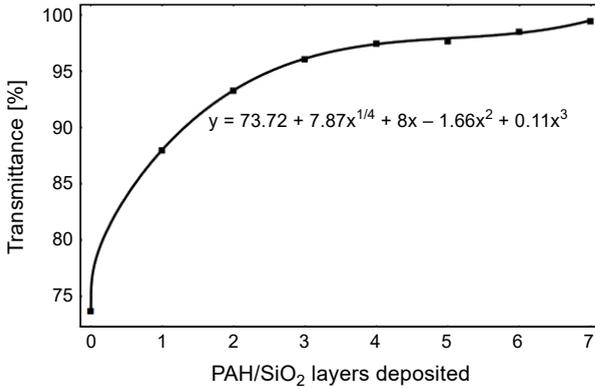
Fig. 3. Transmittance at 611 nm vs. the number of layers deposited.
