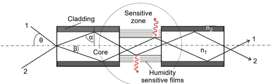
Fig. 1. Ray representation in light propagation along the sensitized FOHS.
