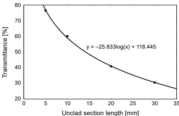
Fig. 2. Transmittance *vs.* the length of the unclad section of the POF.
