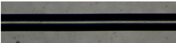
Fig. 1. Photograph of the H-LPFG with a microscope.
