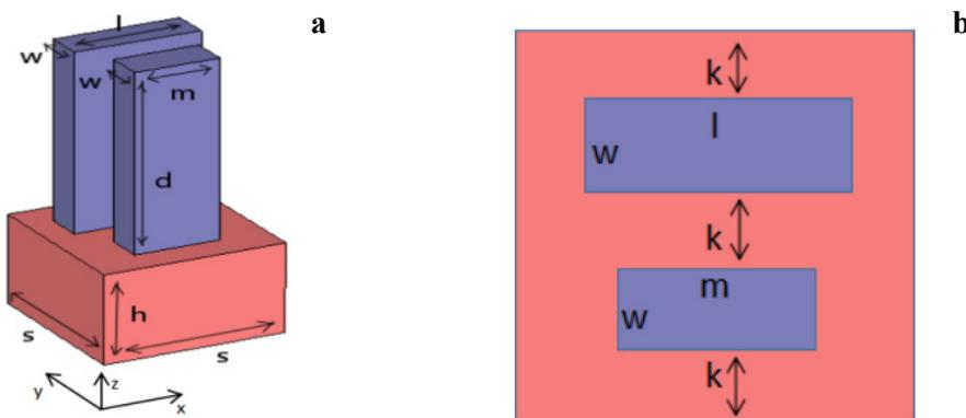
Fig. 2. Schematic diagram of metasurface unit structure.
