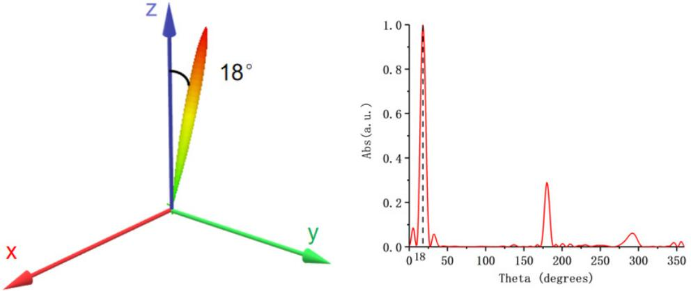
Fig. 8. Scattering angle of the basic sequence S1.
