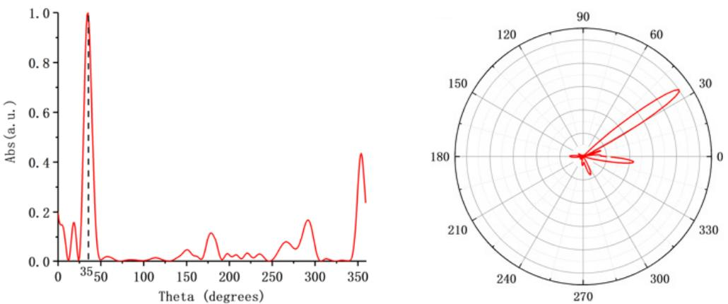
Fig. 37. The scattering results of 450 THz LCP incident on S4.
