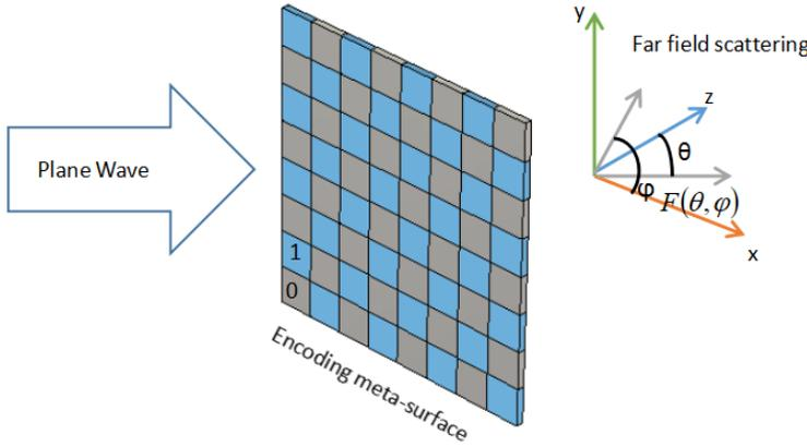
Fig. 1. Schematic diagram of coding metasurface principle.
