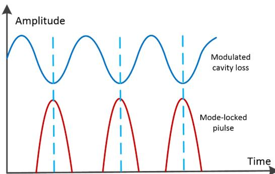
Fig. 3. Schematic diagram of active mode-locking operation.
