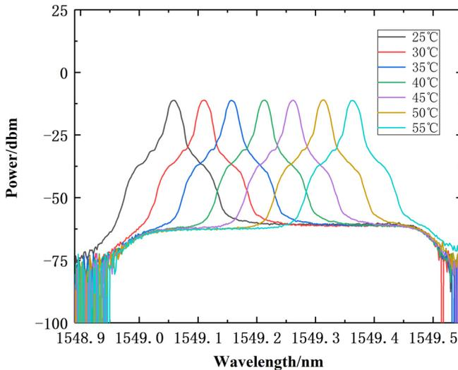
Fig. 8. Laser output spectral lines under different temperatures.
