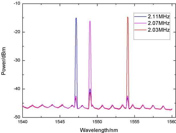
Fig. 6. Spectra observed at different modulation frequencies.
