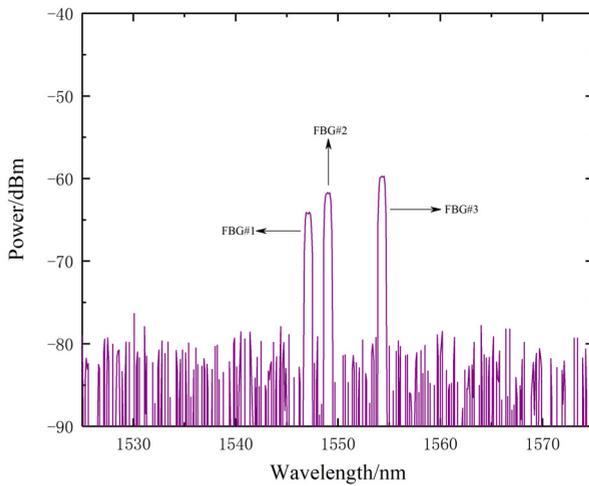
Fig. 4. Spectra of the FBGs under test.
