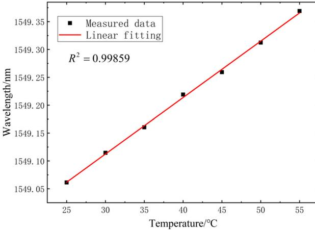
Fig. 9. Fitting line of wavelength at different temperatures.
