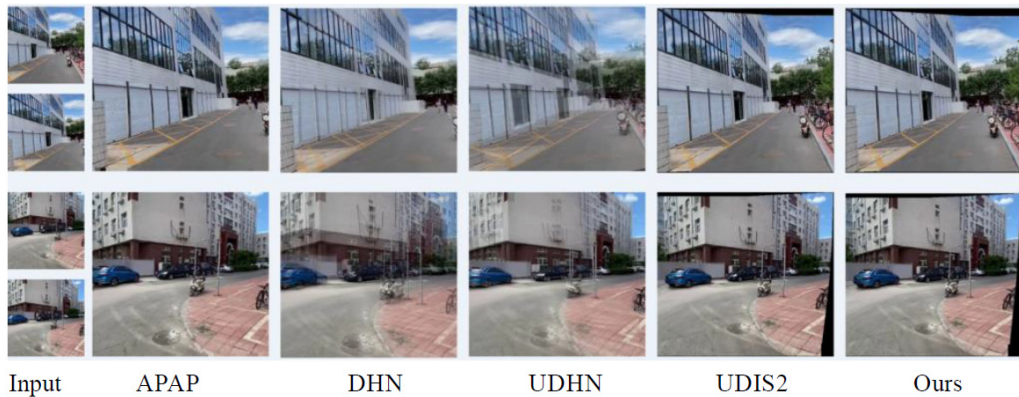
Fig. 4. Visual comparison of stitching results in challenging scenes with large parallax. From left to right: input images, APAP, DHN, UDHN, UDIS2, and our method. Our approach preserves straight-line structures and eliminates ghosting artifacts in overlapping regions.
